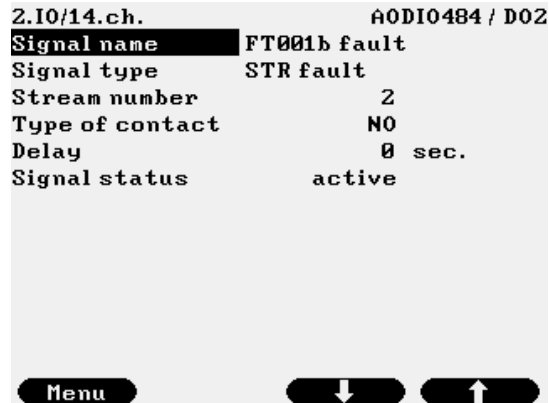
Figure 9-67 Digital output channel (signal type = STR fault alarm) data page
