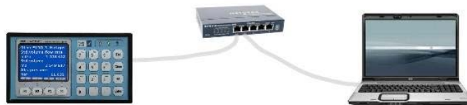
Flow computer – PC Ethernet connection using switch
